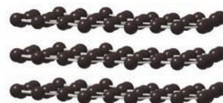
Graphite exists in planar sheets of benzene rings, held together by weak intermolecular forces.
